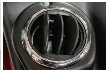
Dashboard with orientable heater outlet
